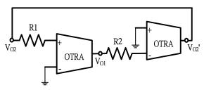
Fig. 2 The quadrature oscillator using OTRAs
