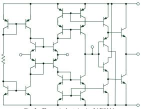
Fig. 5 The equivalent circuit of AD844A
