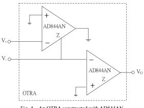
Fig. 4 An OTRA constructed with AD844AN
