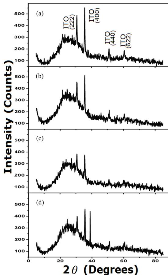
Fig. 4 XRD patterns for (a) ITO/NPB and (b) ITO/NPB/Alq3 heterostructures deposited at  $T_{\text{sub}} = 30^\circ\text{C}$ ; and (c) ITO/NPB and (d) ITO/NPB/Alq3 heterostructures deposited at  $T_{\text{sub}} = 90^\circ\text{C}$
