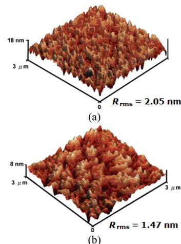
Fig. 1 AFM pictures for ITO substrates (a) as received and (b) post-annealed at  $300^\circ\text{C}$  for 1 h in vacuum
