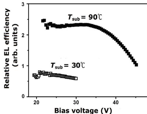
Fig. 6 The values of relative EL efficiency versus bias voltage  $V$  for the ITO/NPB(100 nm)/Alq3(100 nm)/Al OLEDs fabricated at  $T_{\text{sub}} =$  (a)  $30^\circ\text{C}$  and (b)  $90^\circ\text{C}$
