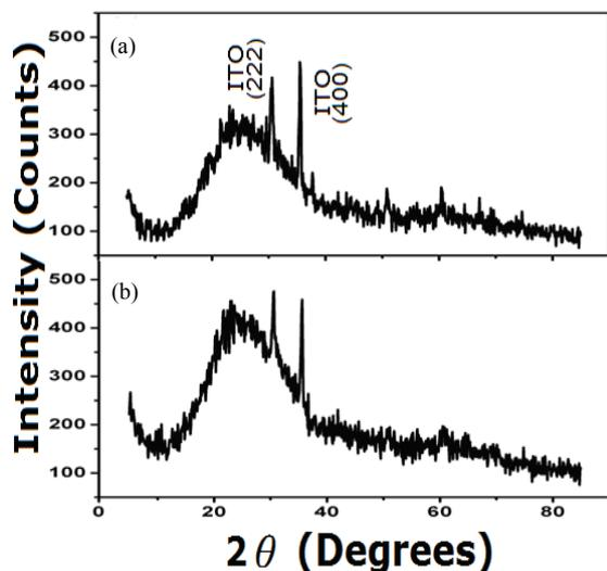
Fig. 2 XRD patterns for ITO substrates (a) as received and (b) post-annealed at  $300^\circ\text{C}$  for 1 h in vacuum
