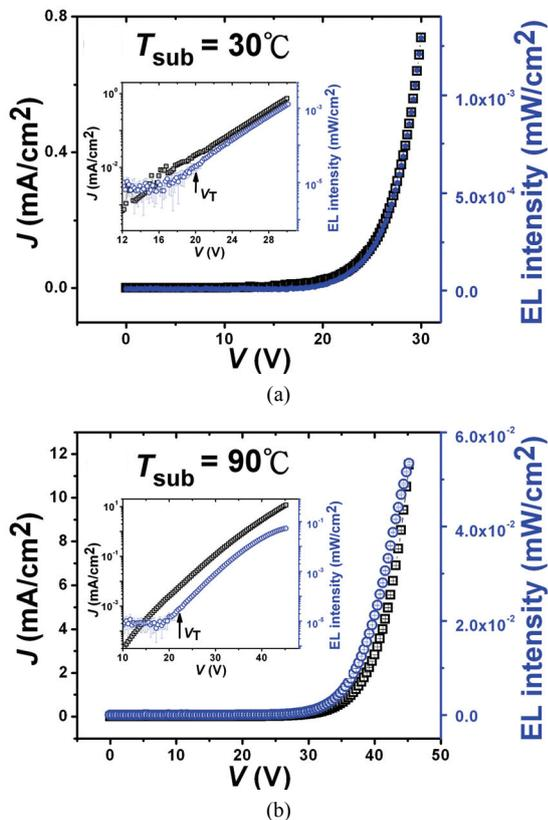
Fig. 5  $J$ - $V$  (with open squares) and  $L$ - $V$  (with open circles) characteristics of the ITO/NPB(100 nm)/Alq3(100 nm)/Al OLEDs fabricated at  $T_{\text{sub}} =$  (a)  $30^\circ\text{C}$  and (b)  $90^\circ\text{C}$
