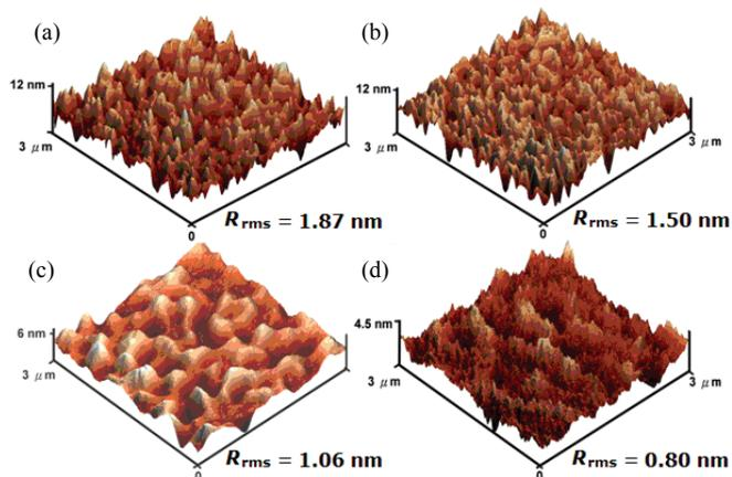
Fig. 3 Surface morphology for (a) ITO/NPB and (b) ITO/NPB/Alq3 heterostructures deposited at  $T_{\text{sub}} = 30^\circ\text{C}$ ; and (c) ITO/NPB and (d) ITO/NPB/Alq3 heterostructures deposited at  $T_{\text{sub}} = 90^\circ\text{C}$
