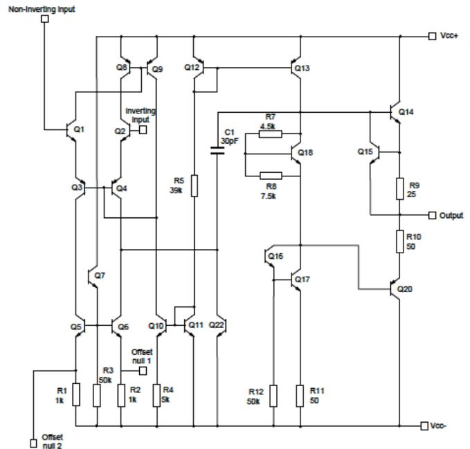
Fig. 6 Detailed schematic of  $\mu A741$
