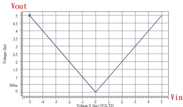
Fig. 1  $V_{out}$  versus  $V_{in}$  transfer characteristic of full-wave rectifier
