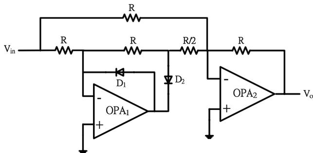
Fig. 2 Simple precision full-wave rectifier for low-frequency operation
