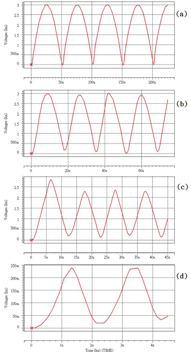
Fig. 11 Output waveforms for the circuit of Fig. 7 to input frequencies (a) 10, (b) 30, (c) 50, (d) 500 kHz
