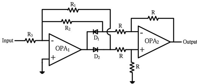
Fig. 3 Precision full-wave rectifier made from a difference amplifier
