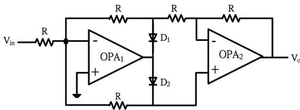
Fig. 4 Another precision full-wave rectifier
