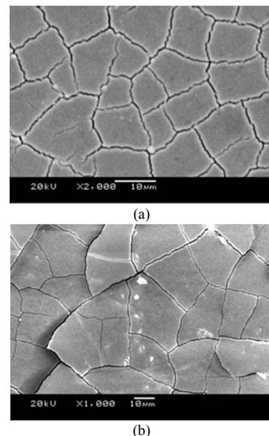
Fig. 4 SEM image showing micrometer grain size of sputtered  $\text{WO}_3$  thin films: (a) as-sputtered condition, and (b) annealed condition
