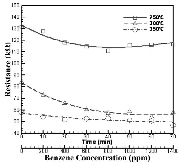
Fig. 8 Sensitivity of benzene sensor as function of working temperature. (Time is measured as the benzene concentration varies.)
