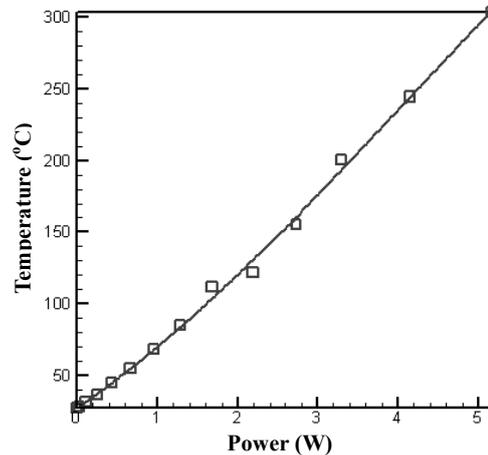
Fig. 7 Variation of micro-hotplate temperature as function of applied power
