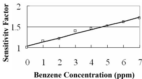
Fig. 10 Sensitivity of benzene sensor at a working temperature of 300°C
