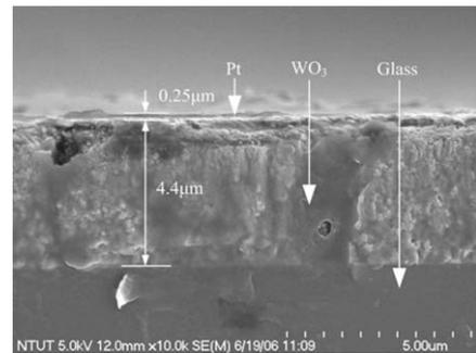
Fig. 3 SEM image showing cross-section of benzene sensor
