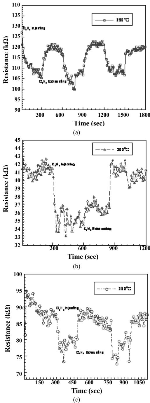
Fig. 12 Repeatability of benzene sensor when benzene concentration is increased from 0 ppm to 200 pm at working temperatures of: (a) 250°C, (b) 300°C, and (c) 350°C.
