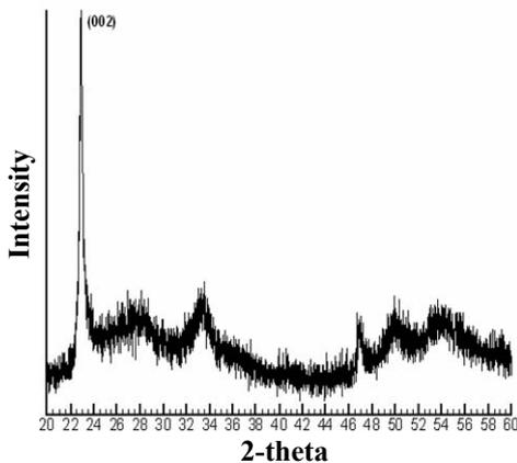
Fig. 6 XRD diffraction pattern of WO<sub>3</sub> film deposited at room temperature. (Note: sputtering conditions as follows: Target, 99.99% WO<sub>3</sub>; RF power of target, 200 W; argon flow rate, 15 sccm; oxygen flow rate, 15 sccm; working pressure, 0.015 torr.)
