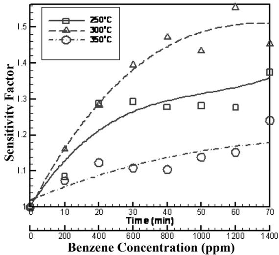
Fig. 9 Variation of sensitivity factor of benzene sensor with benzene concentration as function of working temperature. (Time is measured as the benzene concentration varies.)
