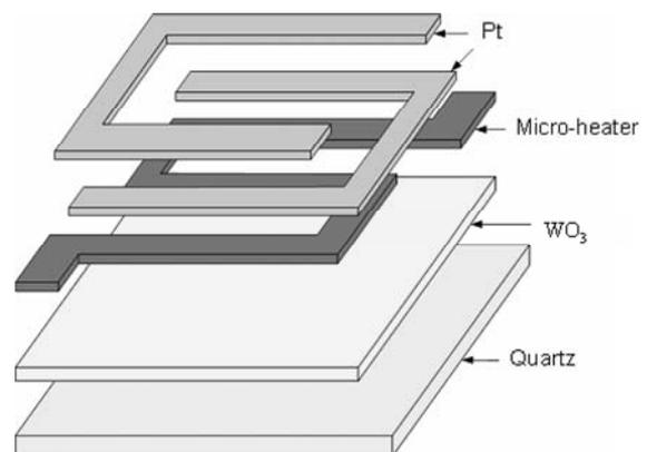
Fig. 1 Schematic illustration of benzene sensor with integrated micro-hotplate and IDEs
