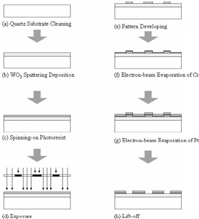
Fig. 2 Overview of fabrication process for  $\text{WO}_3$  thin-film-based benzene sensor
