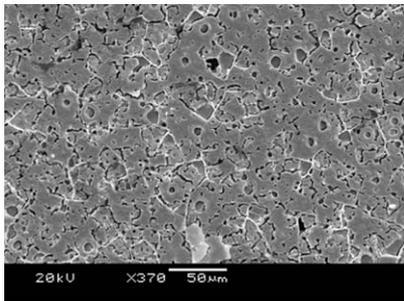
Fig. 5 SEM image showing porous surface of Pt thin film
