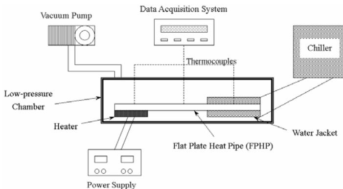
Fig. 1 Schematic of experimental setup
