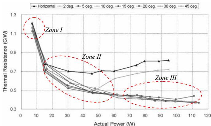
Fig. 7 Thermal resistance of wick FPHP at various inclined angles
