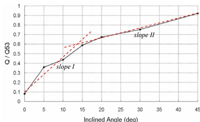
Fig. 4 Normalized maximum heat transfer rate of wickless FPHP at various inclined angles
