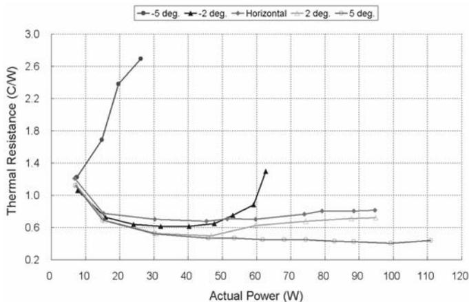
Fig. 6 Thermal Resistance of wick FPHP at small inclined angles
