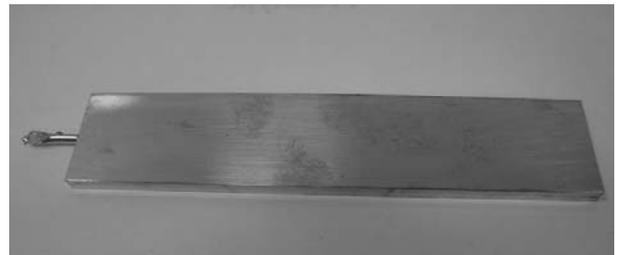
Fig. 2 Prototype of flat plate heat pipe (FPHP)
