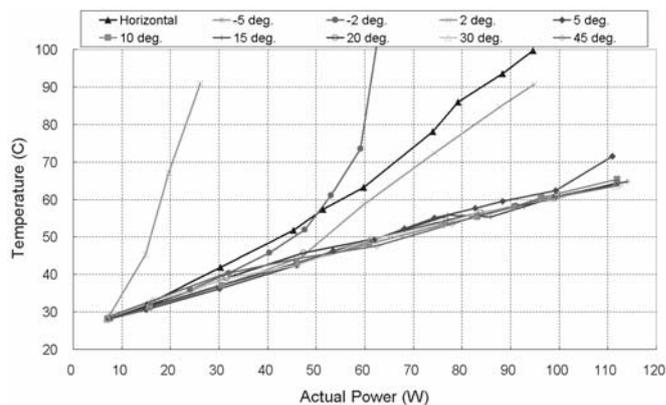
Fig. 5 Heater temperature of wick FPHP at various inclined angles
