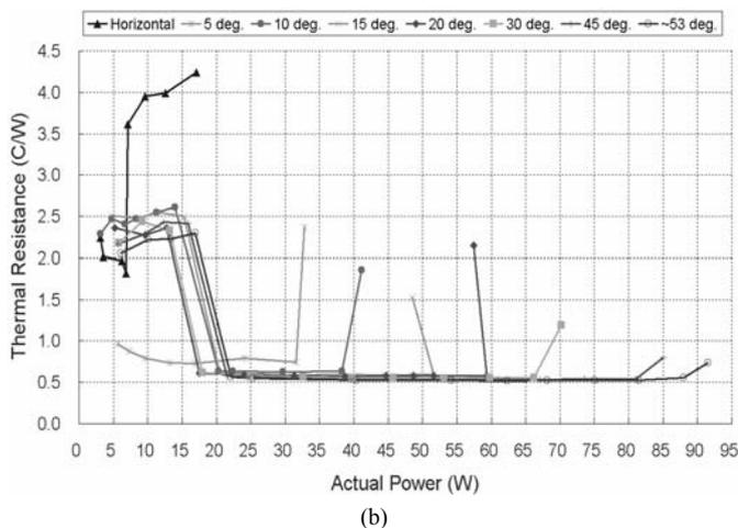
Fig. 3 Thermal performance of wickless FPHP at various inclined angles: (a) heater temperature; (b) thermal resistance
