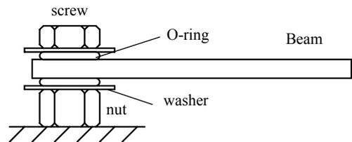
Fig. 3 Beam-support structure
