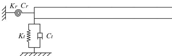
Fig. 2 Schematic diagram of the beam with one-end support
