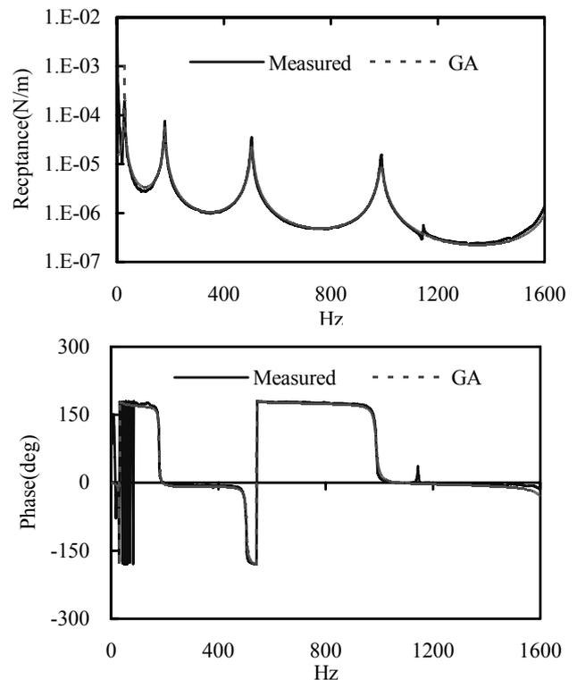
Fig. 8 Comparison of FRFs for  $H_{10\_3}$ , measurement and simulation
