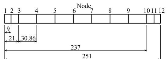
Fig. 4 Finite element modeling of the beam (mm)
