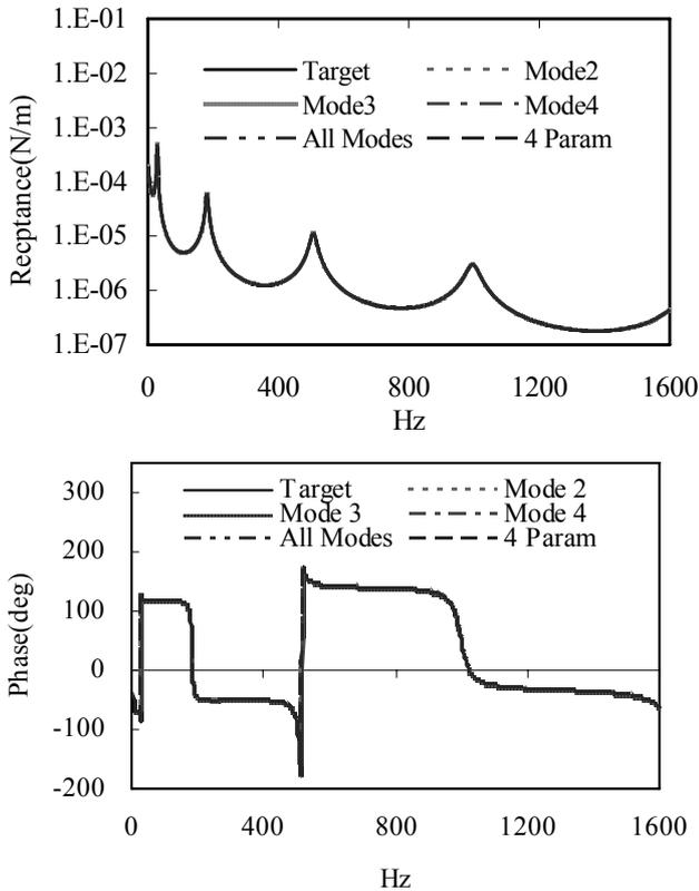
Fig. 7 Comparison of FRFs for  $H_{10\_3}$ , FEM and GA simulation for preset boundary conditions
