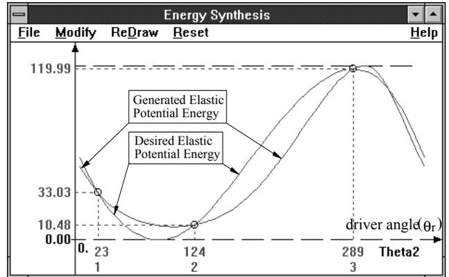
Fig. 14 Elastic potential energies of the first balancer
