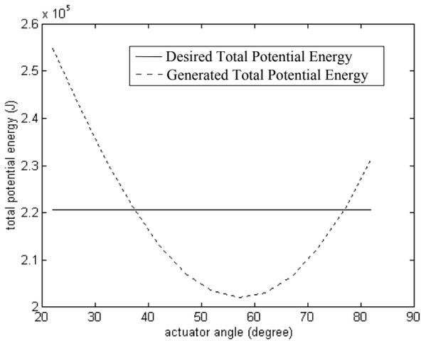
Fig. 11 Desired and generated total potential energies for the elevator
