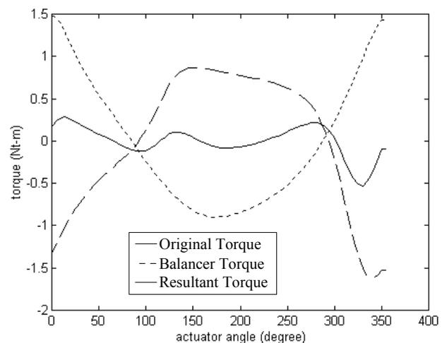
Fig. 19 Torque for superposition example
