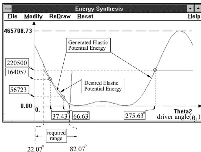
Fig. 9 Elastic potential energies for elevator example
