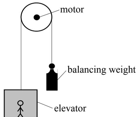
Fig. 6 Elevator with a balancing weight
