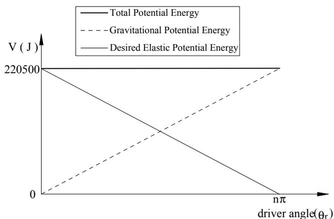
Fig. 7 Energies for elevator example
