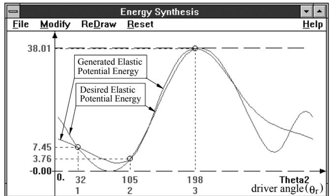
Fig. 15 Elastic potential energies of the second balancer
