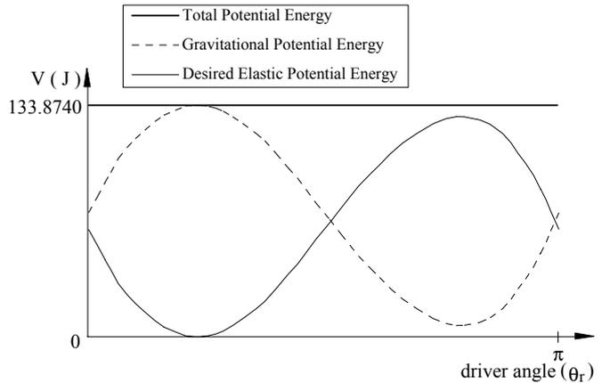
Fig. 13 Energies for superposition example
