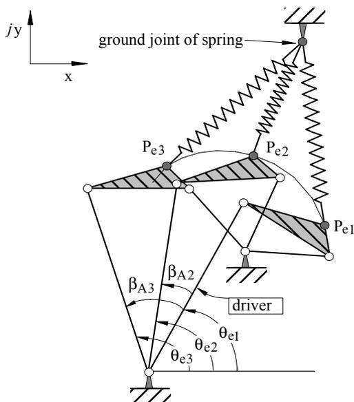
Fig. 4 Three states of the four-bar linkage spring balancer
