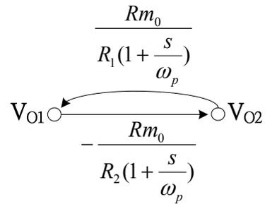
Fig. 3 The signal flow graph for Fig. 2
