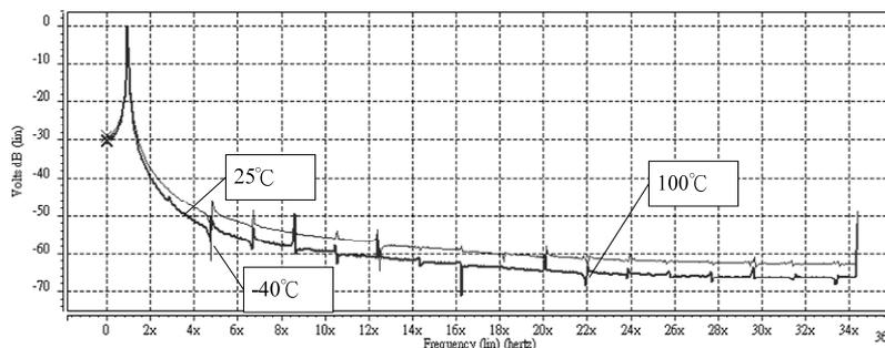
Fig. 7 The frequency spectrum in different temperatures of the OTRA-based oscillator
