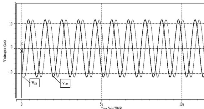
Fig. 6 The output waveforms of the OTRA-based oscillator.
