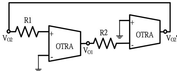
Fig. 2 The quadrature oscillator using OTRAs
