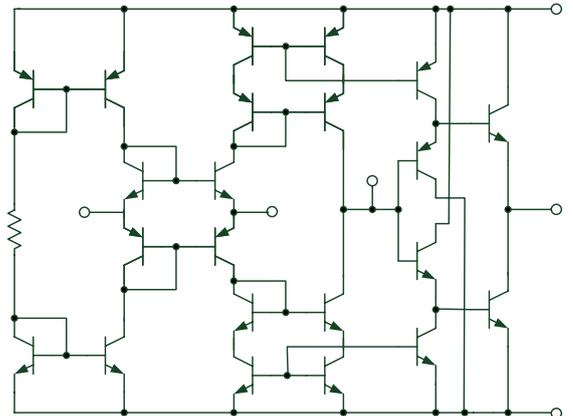
Fig. 5 The equivalent circuit of AD844A
