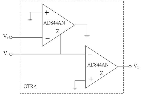
Fig. 4 An OTRA constructed with AD844AN
